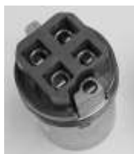
Style 1 Ground conductor attaches to shell.
