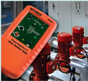
Safe non-contact motor rotation detection
